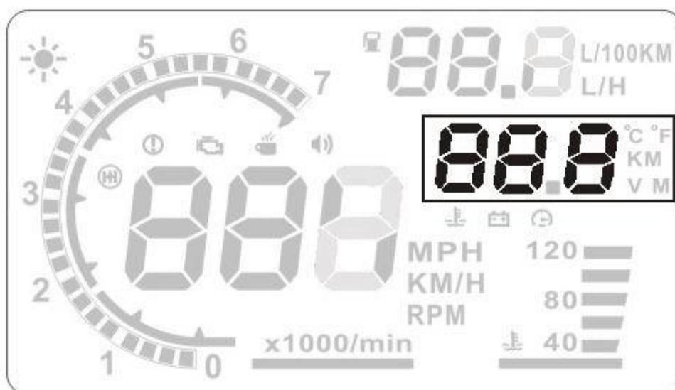
**3. Downturn the wave button for 5 seconds and the alarm buzzer icon will turn off. Upturn the wave button for 5 seconds and the alarm buzzer icon will turn on.**
