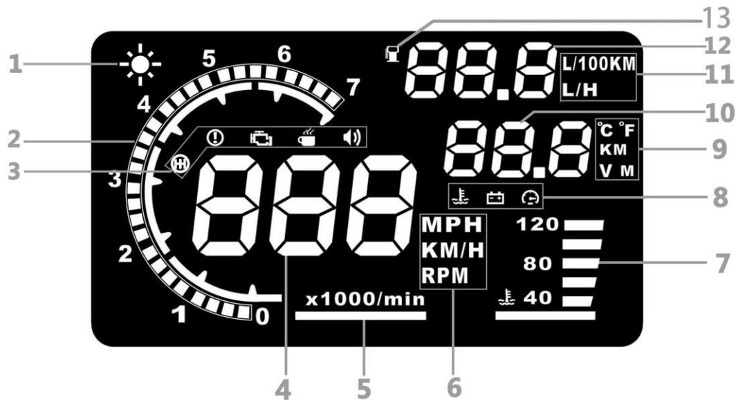
1. Light sensor: Changes the unit's display brightness to suit the constantly changing environment whilst driving.
